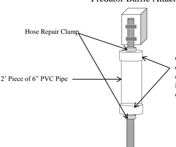
6" PVC End Caps – (You will need to drill a 3/4" hole in center of each end cap so that conduit can slide through it. A larger hole will need to be drilled if you use the T-post.)
